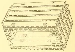
This cut shows a complete Restrictor with the zincs, clamps and reversing wires in use. A large portion of the side sheet is
